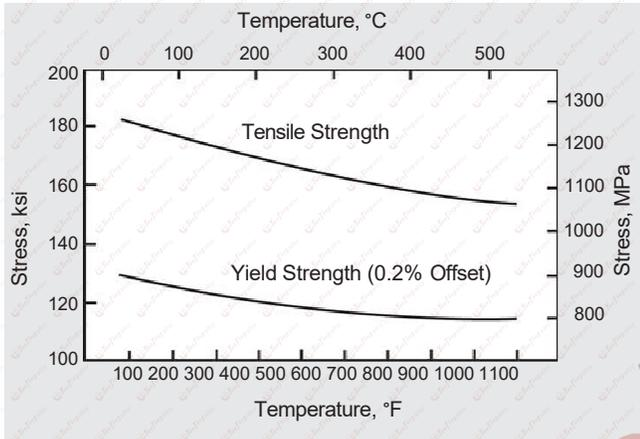
Figure 1. Tensile and yield strength of INCONEL alloy 725.
